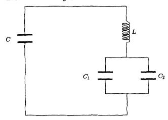
where the most left capacitor C represents a large (parasitic) capacitance. Using Kirchhoff's laws, the dynamics is described by the differential-algebraic equations
